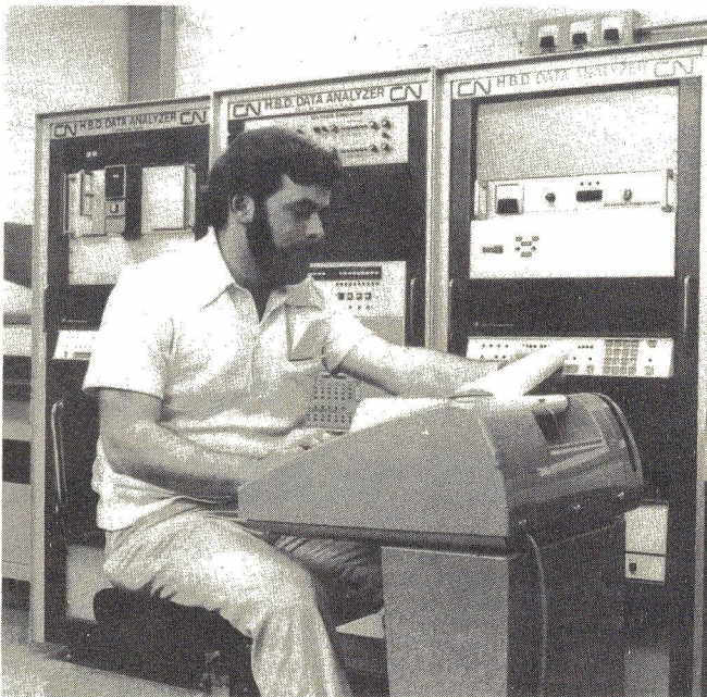
Bryan Smith monitors CN's computerized hotbox detection center at Belleville, Ont., first of its kind in use.
